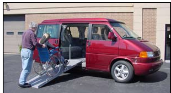
The amount of effort required to lift this AV78 (Aluminum Van Ramp) is under 20 pounds, making it very easy to operate.
