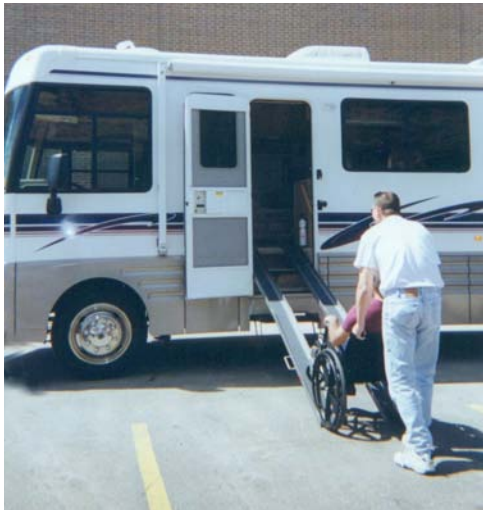
Ten foot long Handi-Traks work with the narrow door of an RV. (Make sure the wheelchair will fit in the door).
