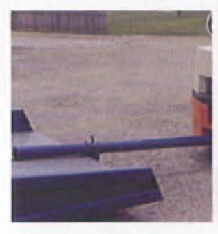
Towbar: The optional towbar features a fast-locking, easy hook-up to the Yardramp and makes towing over long distances practical. A quick disconnect feature improves handling efficiency.
